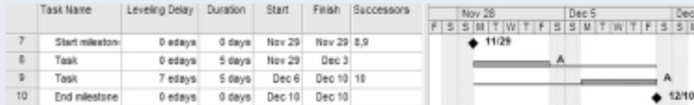
Figure 2 – Both tasks have the same predecessor but one starts later because of leveling delay
